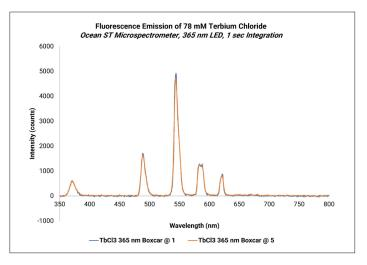
Figure 2. When excited with a  $365\,\mathrm{nm}$  LED, the Terbium chloride solution revealed a strong fluorescence peak near  $550\,\mathrm{nm}$ .
