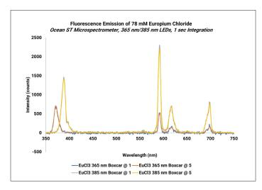
Figure 1. An Ocean ST microspectrometer measures the fluorescence response of Europium chloride. System flexibility allowed us to optimize excitation wavelengths and boxcar averaging.
